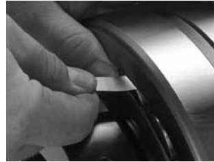
Fig. D-3. Measure RIC before installation.
